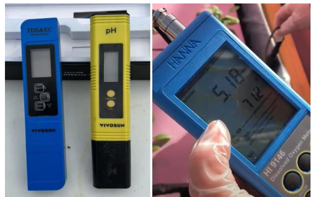
Figure 13. EC and pH meters (left) and DO meter (right). (Toni Sperry, Virginia Tech)
