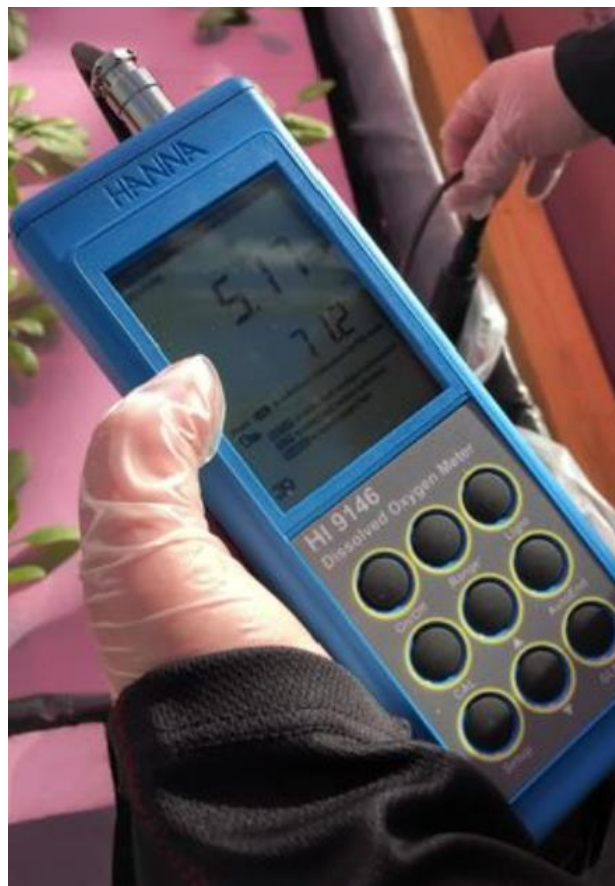
Figure 13. Water nutrient solution from a DWC system being measured using a dissolved oxygen meter (Hanna Instruments, Inc.). (Toni Sperry, Virginia Tech)
