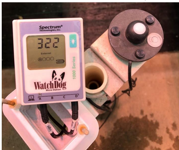
Figure 14. Using a WatchDog (Spectrum Technologies, Inc.) data logger to measure PAR. (Toni Sperry, Virginia Tech)
