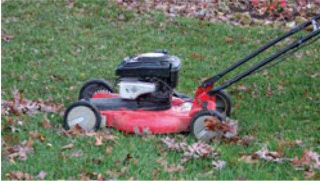
**Figure 3. A mulching mower is an effective tool to chop leaves directly back into the turf canopy without negatively impacting the turf.**
