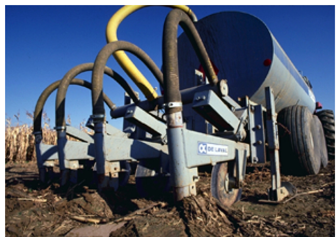
Figure 5. Sub-surface application of liquid manure on land using a slurry tank with injection toolbar to reduce ammonia volatilization.
