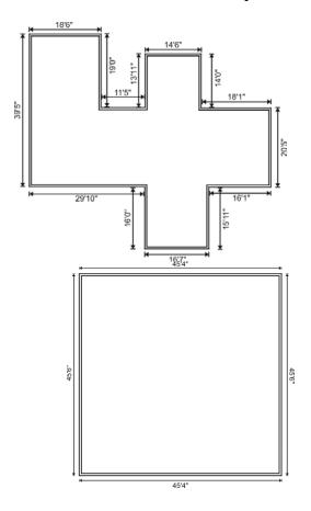
The narrowest parts of the home should be exposed to the east and west (see below). In other words, for optimum efficiency the home should be oriented so that its long axis runs from east to west. This reduces the total amount of surface area exposed to the summer sun, yet when needed in cooler regions, allows the lowangle rays of the winter sun to warm the southern exposure (free solar heating).
