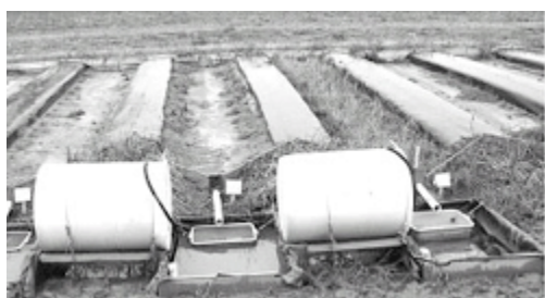
Figure 1. Setup of sedimentation plots. Standard treatment to left, narrow beds in center, and desiccated rye to right.. Photo. taken after 0.3inch rain in September. Note reduced water in tub and box for rye plot
