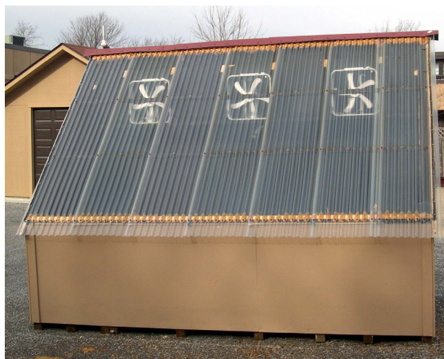
Figure 5. Front view of kiln showing fan placement.
