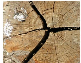
Figure 1. A log with extensive mechanical and biological damage due to improper inventory handling conditions.
