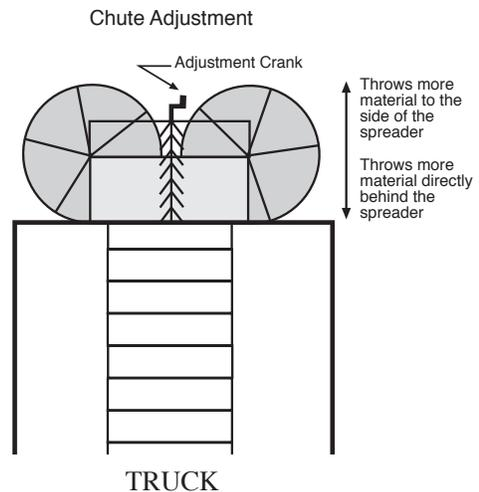
Figure 2. Adjustments for a spreader truck with spinner.
