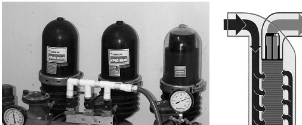
Figure 5. Photo and schematic of disc filter (schematic courtesy of Arkal Filtration Systems).
