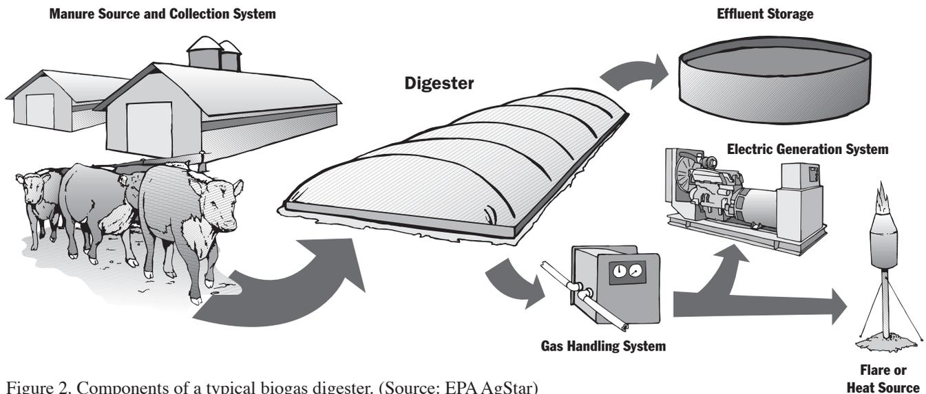
Figure 2. Components of a typical biogas digester. (Source: EPA AgStar)
