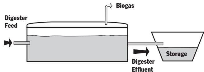
Figure 9. Schematic of a typical plug-flow digester system.
