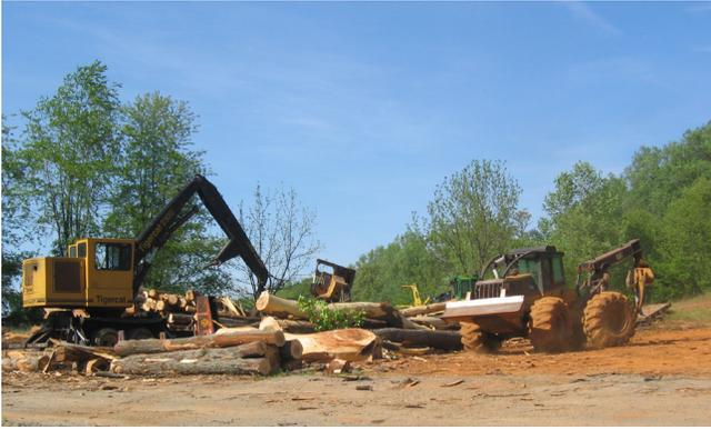
A log loader is stationed on the log deck and is used to load the sorted logs onto trucks. Sometimes logs are sorted for going to different mills, and the loader may also be equipped to delimb trees and cut them to length.
