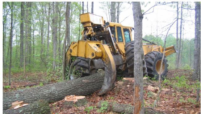
After trees are either felled with a piece of machinery or by hand with a chainsaw, they are typically moved to the log deck with a skidder, such as this “grapple”-style skidder that lifts one end of the log and drags the other.
