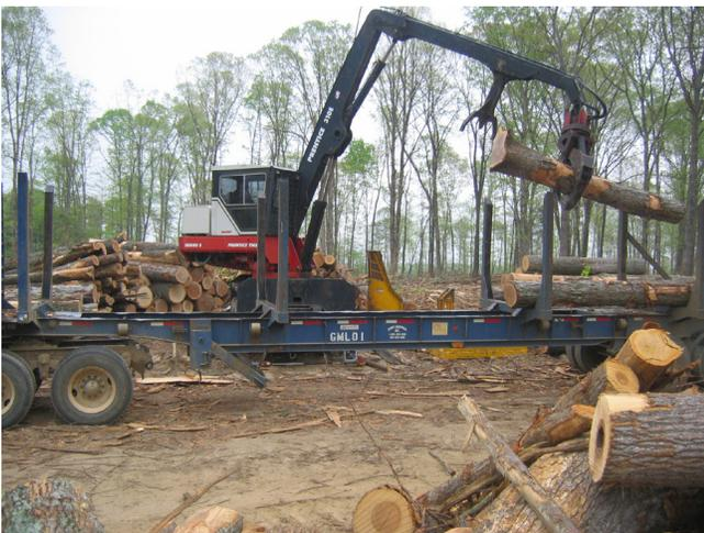
A log deck is an area of high activity and high impact where logs are concentrated, sorted, and loaded onto trucks.
