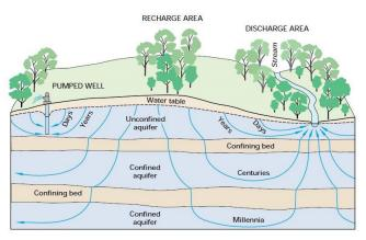
Figure 4. Travel times for groundwater along different flow paths. (Source: Winter et al. 1998)
