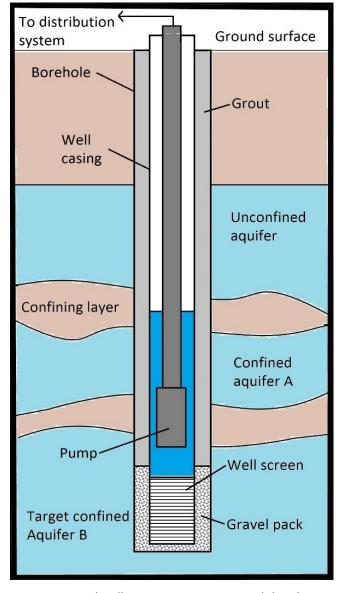
Figure 6. Typical well construction in unconsolidated material (not to scale). (Adapted from VDEQ 2014)
