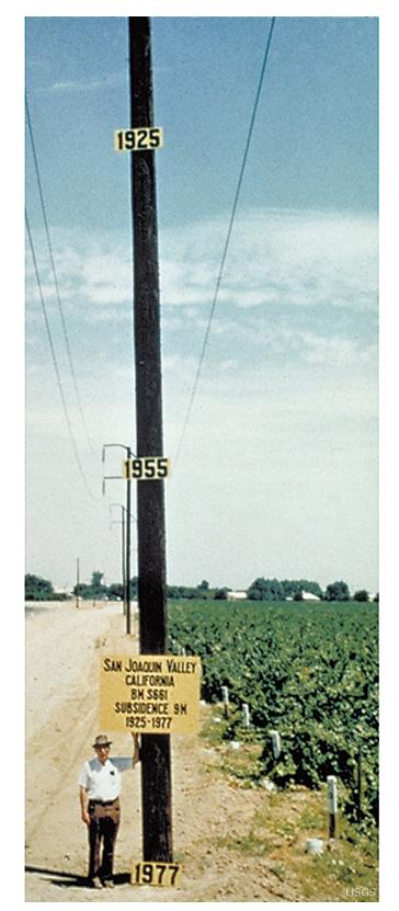
Figure 5. Signs on a telephone pole show how much the land subsided in the San Joaquin Valley between 1925 and 1977. (Source: USGS 2000b)
