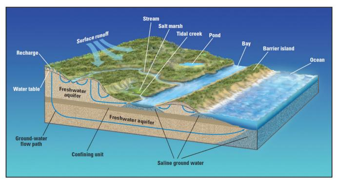
Figure 2. The movement of water between surface and subsurface features. (Source: Barlow 2003)
