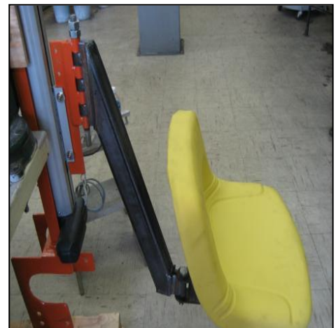
Complete vertical lift assembly on support structure (picture in a machine shop).
