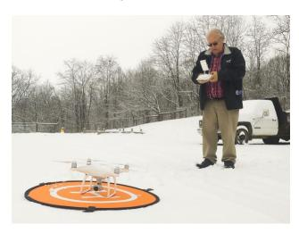
Figure 1: Using a landing pad like the one pictured reduces the drone's contact with moisture during takeoffs and landings.
