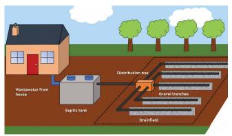
**Figure 2:** Effluent leaves the septic tank and is distributed through the drainfield via a distribution box. Effluent is treated as it passes through the soil profile.
