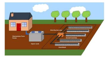
Figure 2. Effluent leaves the septic tank and is distributed through the drainfield via a distribution box. Effluent is treated as it passes through the soil profile.
