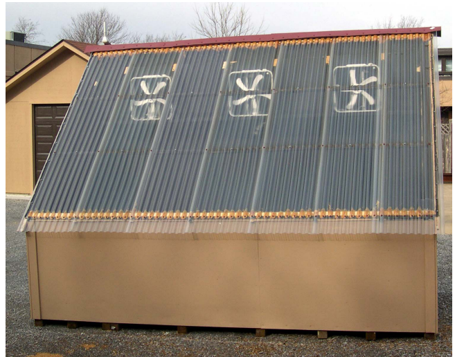
Figure 5. Front view of kiln showing fan placement.
