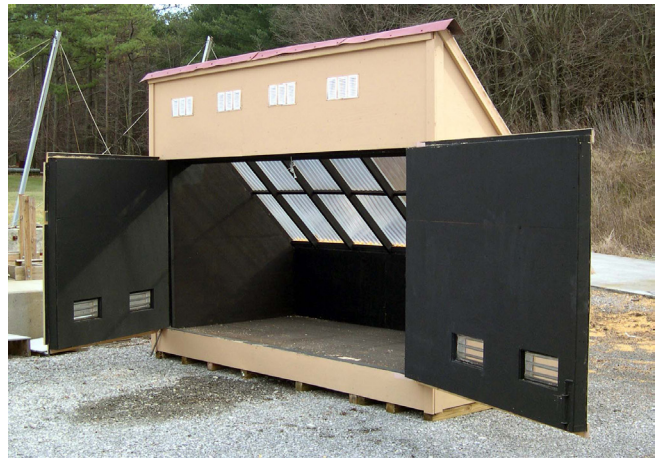
Figure 4. Rear view of kiln showing access doors.
