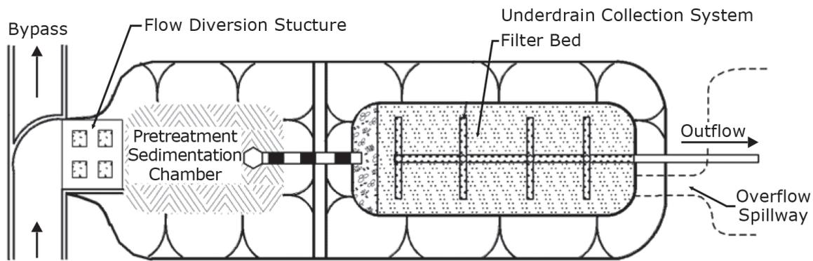
Figure 2. Plan view of typical filtration practice.
