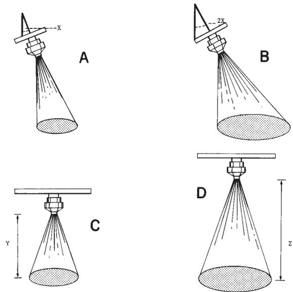
**Figure 3.** (A) and (B) show how the angle of the spray pattern affects the width of the pattern. As the angle,  $x$ , is increased from (A) to  $2x$  in (B), the pattern width increases proportionately. The height of the nozzle above the ground also affects the width of the spray pattern, as shown in (C) and (D). As the height,  $y$ , in (C) increases to a height of  $z$  in (D), the pattern width increases proportionately.
