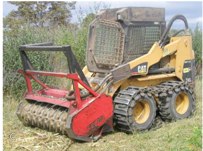
Figures 3a - c. Equipment that can be used for site clearing operations: (a, upper left) a “KG-style” shearing blade, attached to a dozer, for shearing dense woody vegetation at ground level; (b, lower left) a brush-rake, also attached to a dozer, for grubbing roots and moving and piling sheared vegetation with low disturbance of surface soils; and (c, upper right) a tree shredder, attached to a skid-steer tractor, for grinding and shredding both above-ground and below-ground stumps and roots, an operation that can prevent much of the vigorous re-sprouting that will occur if only woody tops are removed.
