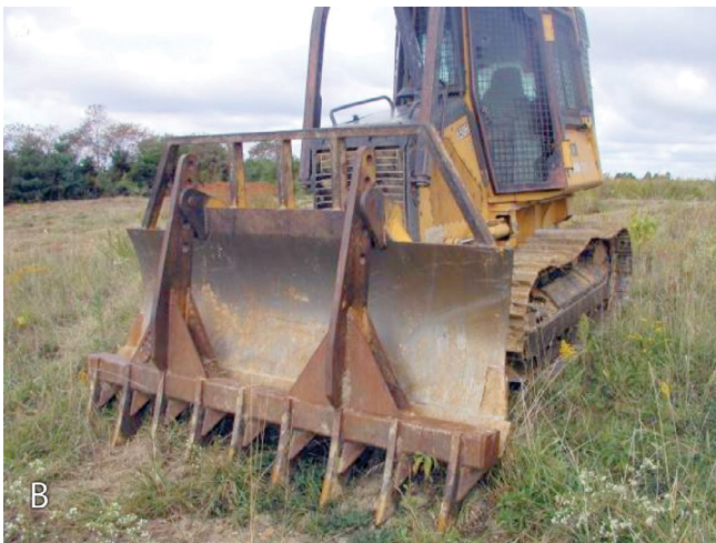
Figures 3a - c. Equipment that can be used for site clearing operations: (a, upper left) a “KG-style” shearing blade, attached to a dozer, for shearing dense woody vegetation at ground level; (b, lower left) a brush-rake, also attached to a dozer, for grubbing roots and moving and piling sheared vegetation with low disturbance of surface soils; and (c, upper right) a tree shredder, attached to a skid-steer tractor, for grinding and shredding both above-ground and below-ground stumps and roots, an operation that can prevent much of the vigorous re-sprouting that will occur if only woody tops are removed.
