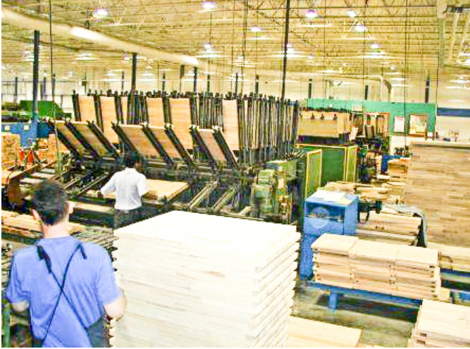
Figure 9. A hardwood panel gluing operation. Photo credit: Urs Buehlmann.
