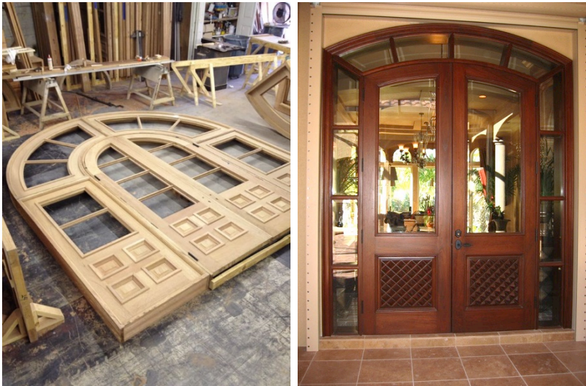
Figure 10. Custom-made entry doors, in process (left) and installed (right), are a value-added wood product. Photo credit: Diana Mourin-Ayish.
