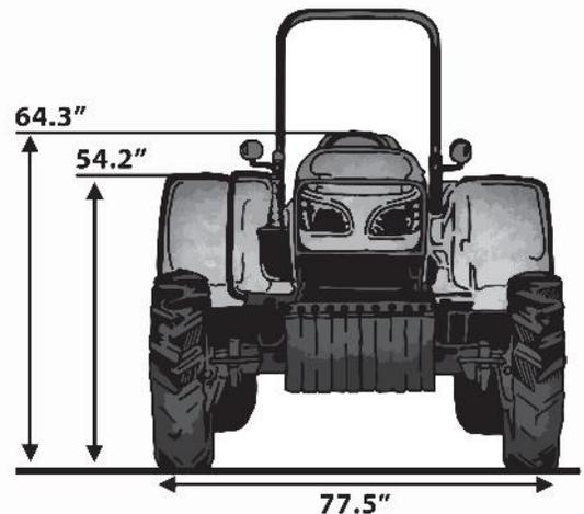
Figure 4. A low-profile tractor with ROPS (<http://www.kubota.com/product/M40LOW/M40LowProfile.aspx?tab=lowprofile>)
