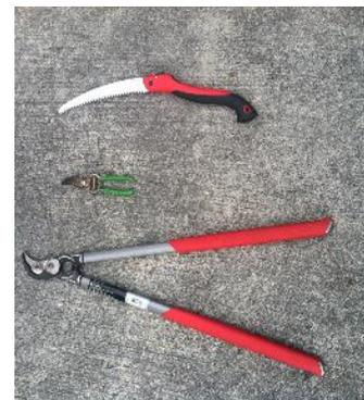
Figure 1. Other tools used for pruning. From top to bottom Saw, hand shears, and lopping shears.
