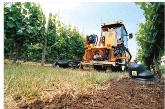
Figure 18. Tournesol mechanical weeder
