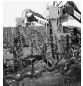
Figure 10. Korvan vineyard mechanization system shear pruner (Morris, 2007)
