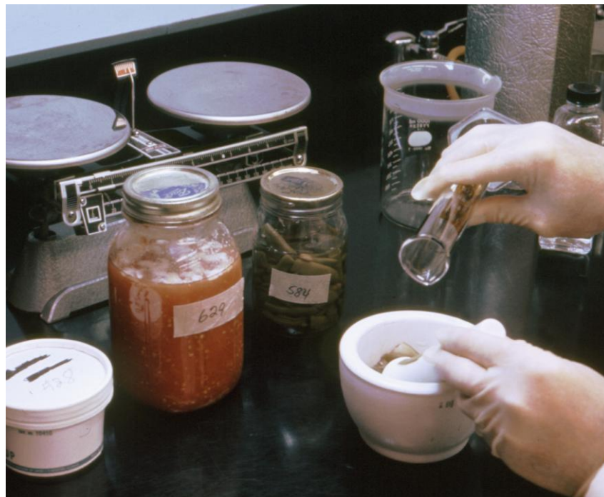
Canned food samples are prepared to be tested for the toxin produced by Clostridium botulinum . Photo courtesy of the Center for Disease Control and Prevention (CDC).
