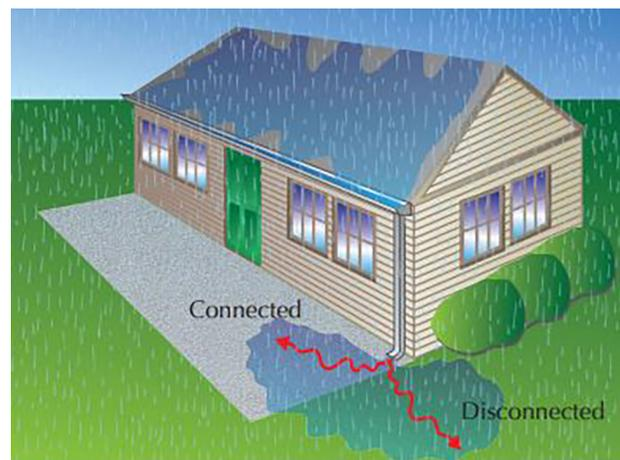
Figure 1. Diagram of water flow with rooftop redirection.
